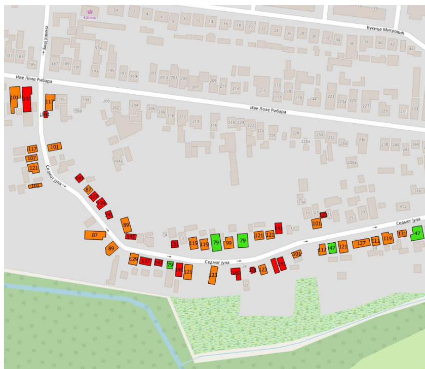
Figure 24. Structural vulnerability of 50 houses in the 7. Jula Street in Bačka Palanka urban settlement in the case of a windstorm hazard. Each color and number represents the degree of structural vulnerability. Data was obtained from Google Street View imagery from September 2014.
