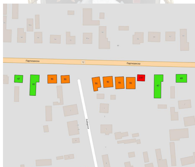
Figure 25. Structural vulnerability of randomly chosen 11 houses in the Partizanska Street in the Begeč rural settlement in the case of windstorm hazard. Each color and number represents the degree of structural vulnerability. Data were obtained through a field observation survey conducted on the ground on 8 February 2026.
